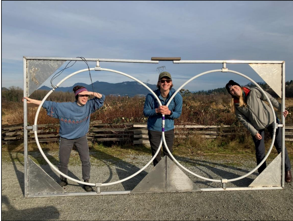
Figure 5: Front on perspective of innovative infinity loop PIT antenna design. Photo by: Zachary Sherker, project lead
