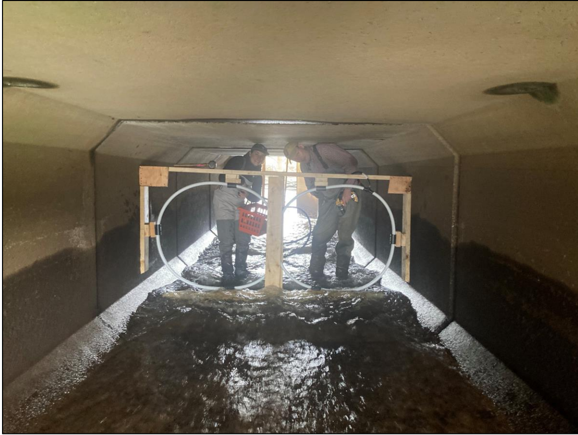
Figure 9: Antenna setup inside Sheep Paddocks control site. Photo by Zach Sherker
